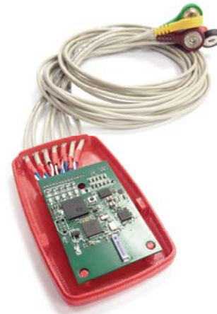
Fig. 5. The ECG module with the respiration impedance measurement.
