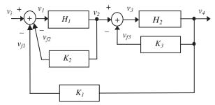
Fig. 7. Modified structure of Fig. 4 with a feedback connection of two nonlinear circuit basic blocks denoted as  $H_1$  and  $K_2$  instead of a basic block denoted as  $H_1$  in Fig. 4.
