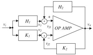
Fig. 8. Circuit structure using op amp as a basic element three-terminal element and with two feedback loops associated with its inverting and non-inverting inputs.
