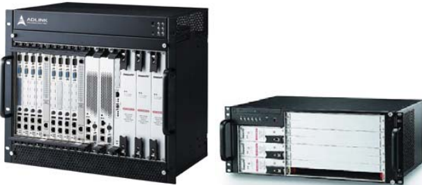
Fig. 1. The ATCA shelves for ATCA Carrier boards (left) and \mu TCA cards [14].
